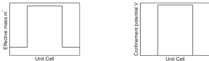
Figure 4.6. Effective mass and confinement potential in the fine scale unit cell. ( See also Color Plate on page 369 )
