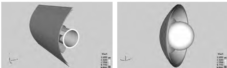
Figure 5.6. Mach isosurfaces for flow past a cylinder, third order reconstruction (left) and past a sphere, second order reconstruction (right). (See also Color Plate on page 376)
